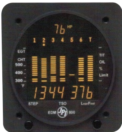
A non-firing spark plug or faulty ignition lead affects only one cylinder, while a faulty mag affects all cylinders.
