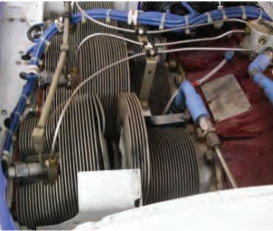
Figure 3—Head-to-barrel separation of the No. 5 cylinder on a Continental TS10-520 engine.
