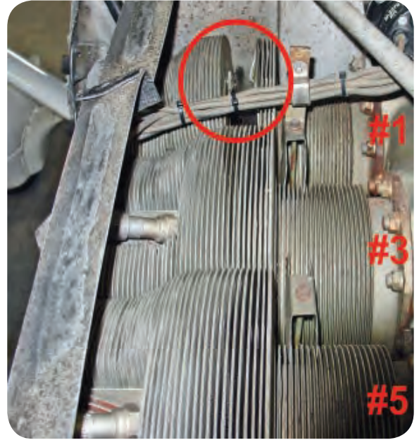
Figure 1—The No. 1 cylinder head on this TCM O-470-U engine suffered a catastrophic fatigue failure in flight. The No. 3 cylinder suffered a similar failure about an hour later.
