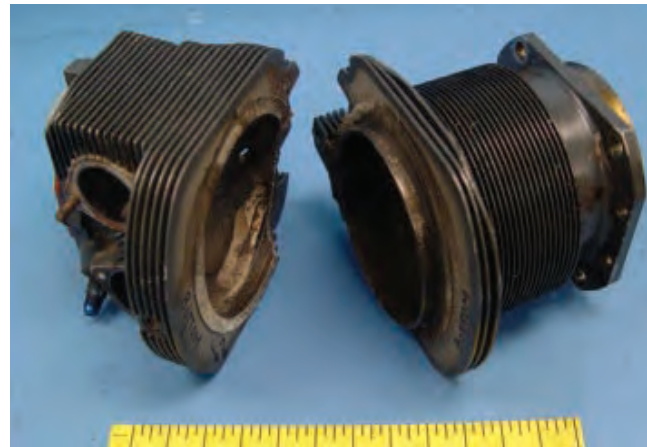
Figure 2—Head-to-barrel separations are not limited to Continental engines. Here's a Lycoming cylinder that lost its head.
