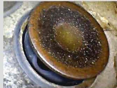
LYCOMING O-320 exhaust valve. Note the symmetrical "bullseye" appearance indicating a healthy valve.
