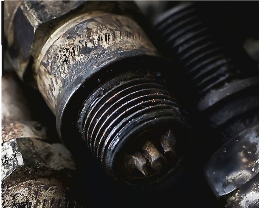
AN A&P may clean the spark plugs and perform other tasks in an attempt to resolve a problem such as partial power loss—but confirmation of the root cause may be elusive.
