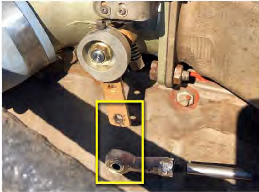
THE THROTTLE CABLE was found disconnected from the throttle bellcrank, and the attaching hardware was gone.
