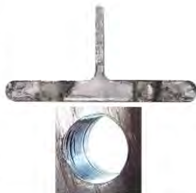
FRACTURE SURFACE (TOP) of failed PA-28 left wing lower spar cap that fractured through the outboard bolt holes. Corresponding right-wing bolt holes exhibited cracking caused by repetitive bearing stress (bottom). This was a high-time airplane with a history of hard landings and high load-factor maneuvers.
