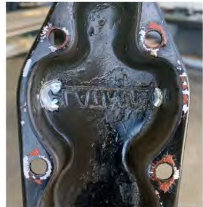
INSIDE OF VALVE COVER gouged by loose bolts to the point of cracking and leaking oil.
