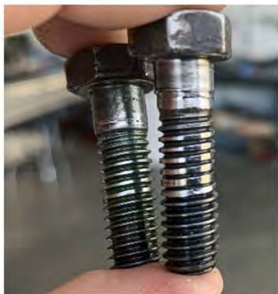
LOOSE BOLTS were badly stripped and stretched.
