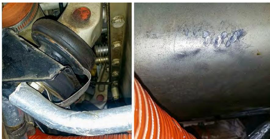
**SAGGING VIBRATION** isolators (left) resulted in severe chafing that gouged grooves into the engine's oil sump (right).
