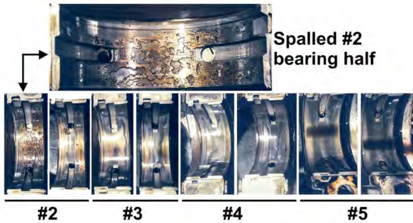
THE ENGINE SHOP tore down Frank's engine and found one half of the number 2 main bearing exhibited serious spalling.
