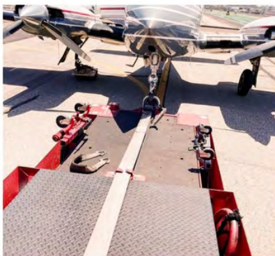
Recovery as viewed from Lektro tug, with axle lashed to dolly.
