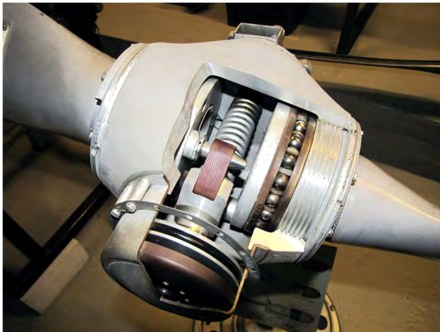
The hub of a constant-speed prop contains stuff that your IA cannot inspect. A reseal repair is the most economical way to deal with that.
