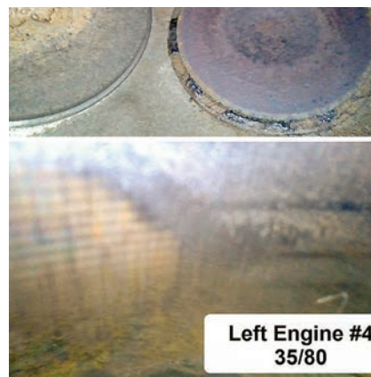
Left engine cylinder number 4, compression is 35/80.
