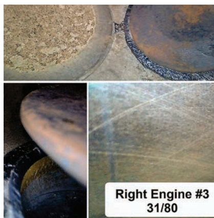
Right engine cylinder number 3, compression is 31/80.
