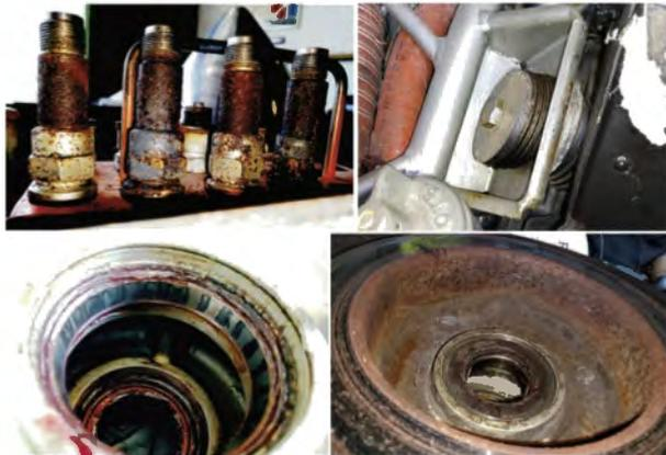
Some prebuy lowlights: rusted spark plugs, sagging engine shock mounts, rusted and warped brake disc, bad wheel bearings.
