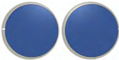
Ring gap position can profoundly affect compression readings. (Dimensions are exaggerated here to help illustrate the issue.)
