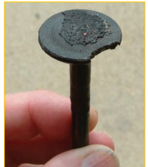
Exhaust valves often don't survive to TBO. If we don't catch a potential exhaust valve failure using compression tests, borescope inspections, and engine monitor data, we risk a total failure ("swallowed valve").
