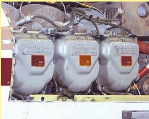
On this big Continental six-banger, mechanics have made note of the compression readings of each cylinder over the years—showing as low as 50/80 pounds at one time. The most recent readings, noted in fresh Sharpie ink, are all in the healthy 70s.
