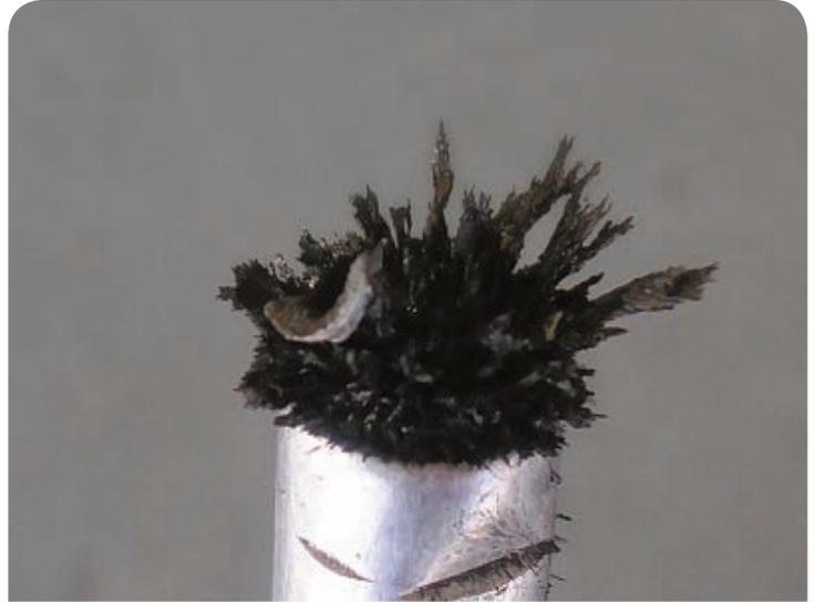
*Running a mechanic's magnetic pickup tool around in the drained oil is a good idea for any engine, but particularly for Continental engines where the suction screen cannot be inspected.*
