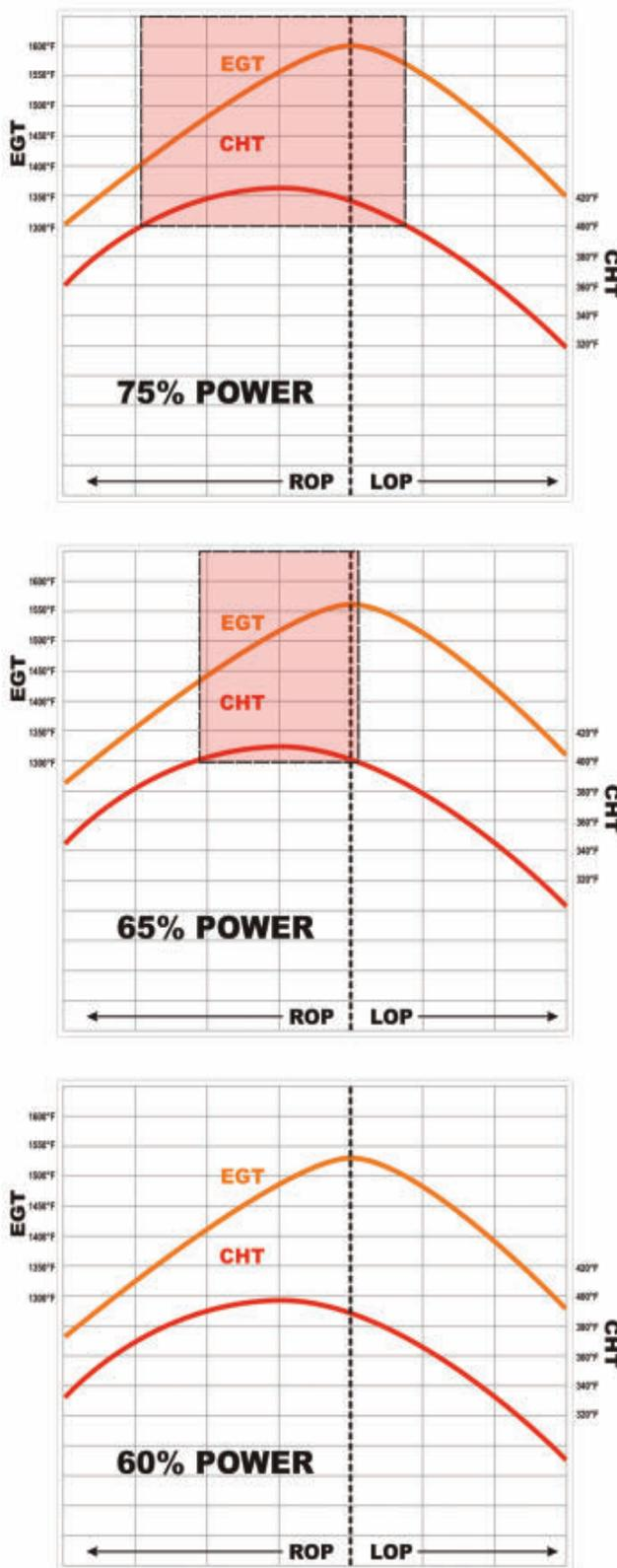
Figure 1—The lower the power, the narrower the red box becomes. Somewhere between 60 percent and 65 percent for most engines, it disappears completely.
