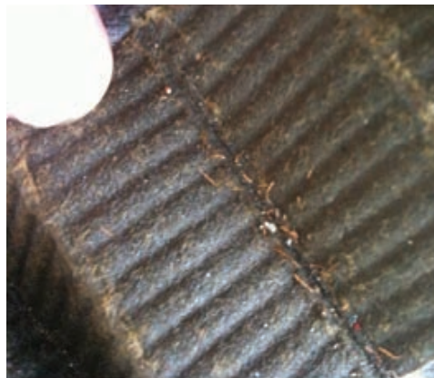
Figure 2—How is a mechanic to determine how much metal in the oil filter is too much?
