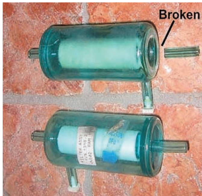
Figure 3—Fracture of this plastic magneto pressurization filter caused simultaneous and severe high-altitude misfire of both magnetos. So much for redundancy...
