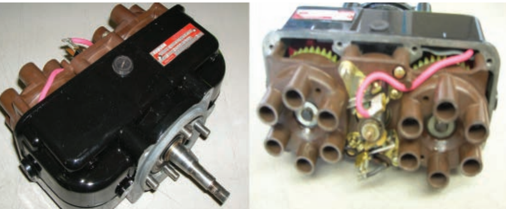
Figure 2—The Bendix D2000/D3000 dual mag is basically two independent magnetos packaged into a single unit.
