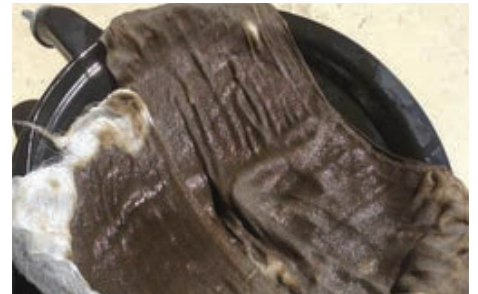
Mark strained his engine oil through cheesecloth to make sure the little chunk of aluminum found in his oil pressure relief valve "didn't have a bunch of brothers and sisters floating around in the oil pan."
