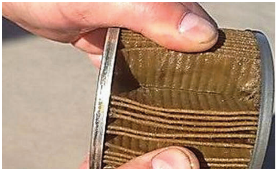
After a 30-minute ground run and a full-power high-speed taxi run, the oil filter was spotless.
