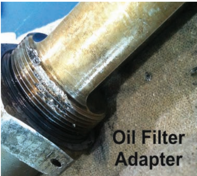
Source of the aluminum chunk found in the pressure relief valve: torn-up threads in the oil pump caused by a loose oil filter adapter. Mystery solved!
