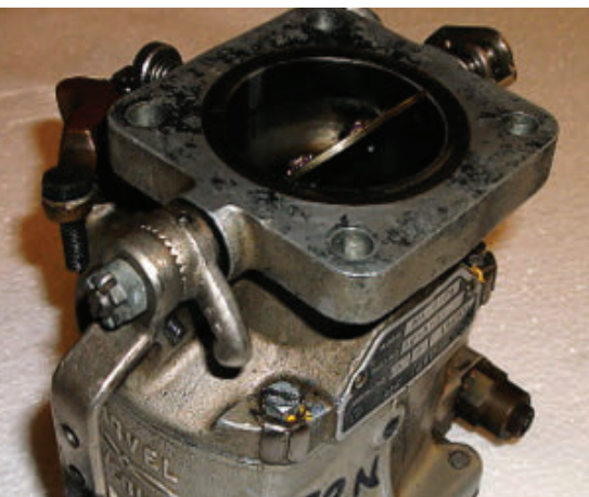
The O-320's carburetor was re-jetted to increase takeoff fuel flow from 12.5 to 13.5 gph.
