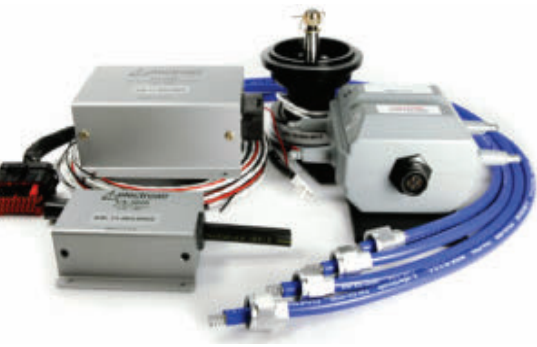
The O-320's right magneto was replaced with an Electroair electronic ignition system.
