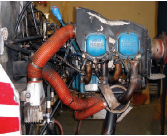
The 1976 Skyhawk's original 150-hp Lycoming O-320-E2D engine and 53-inch pitch prop was modified with a high-compression piston STC and a 57-inch pitch prop STC to produce 160 hp.
